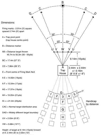
of A: 2.44m (8') to 3.05m (10') above the level of Firing Mark No3
